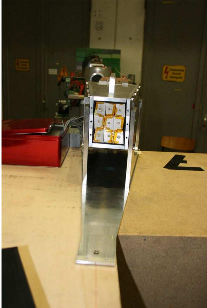
Figure 4.4: A  $3 \times 3$  matrix in the beam line seen downstream from behind the MiniTAPS detector. In this particular measurement the upper left crystal was aligned centrally in the beam.
